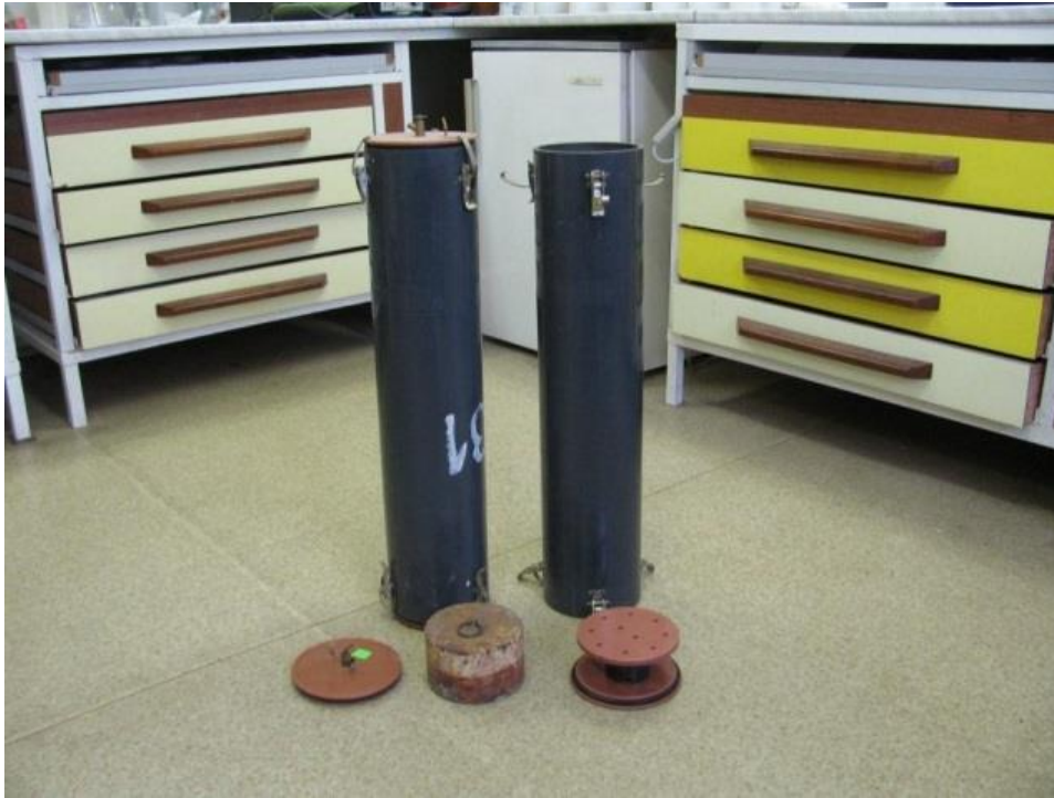
Photo 1 plastic laboratory mini-silos for fermentation of silage, with a double bottom and weight
